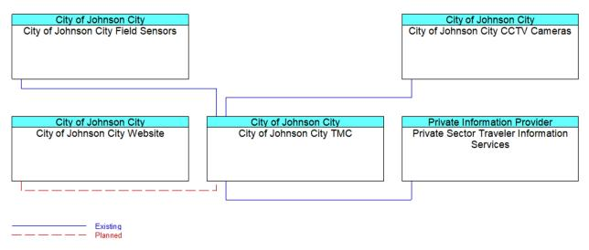
Figure 5 – Example Interconnect Diagram: City of Johnson City TMC
